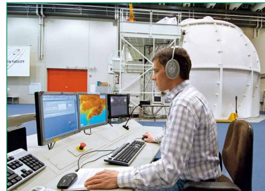
The FMS instructor station, where simulated missions can be planned – or the pilot can be confronted with an unexpected engine failure
