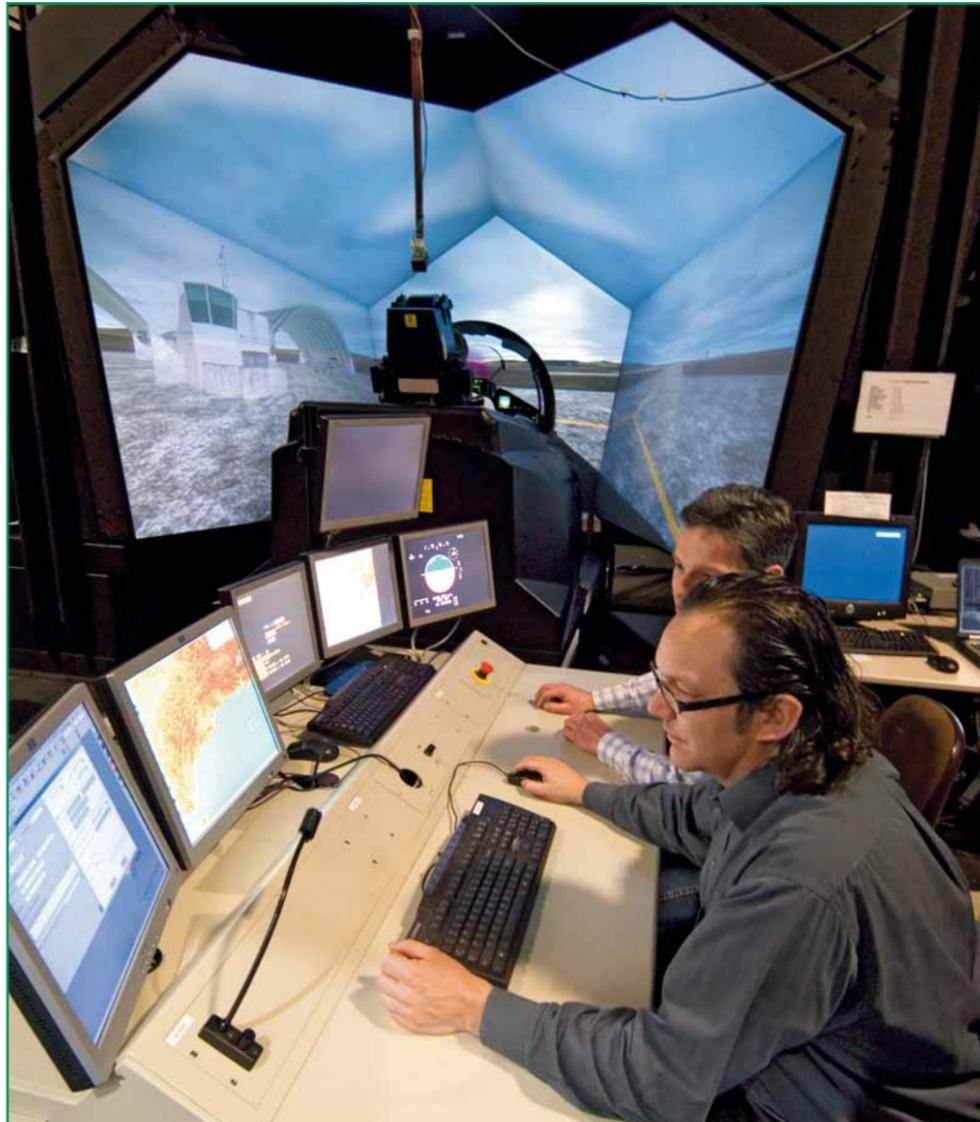
The Cockpit Trainer instructor station. The trainer is used primarily for basic Eurofighter orientation and instruction in emergency procedures
